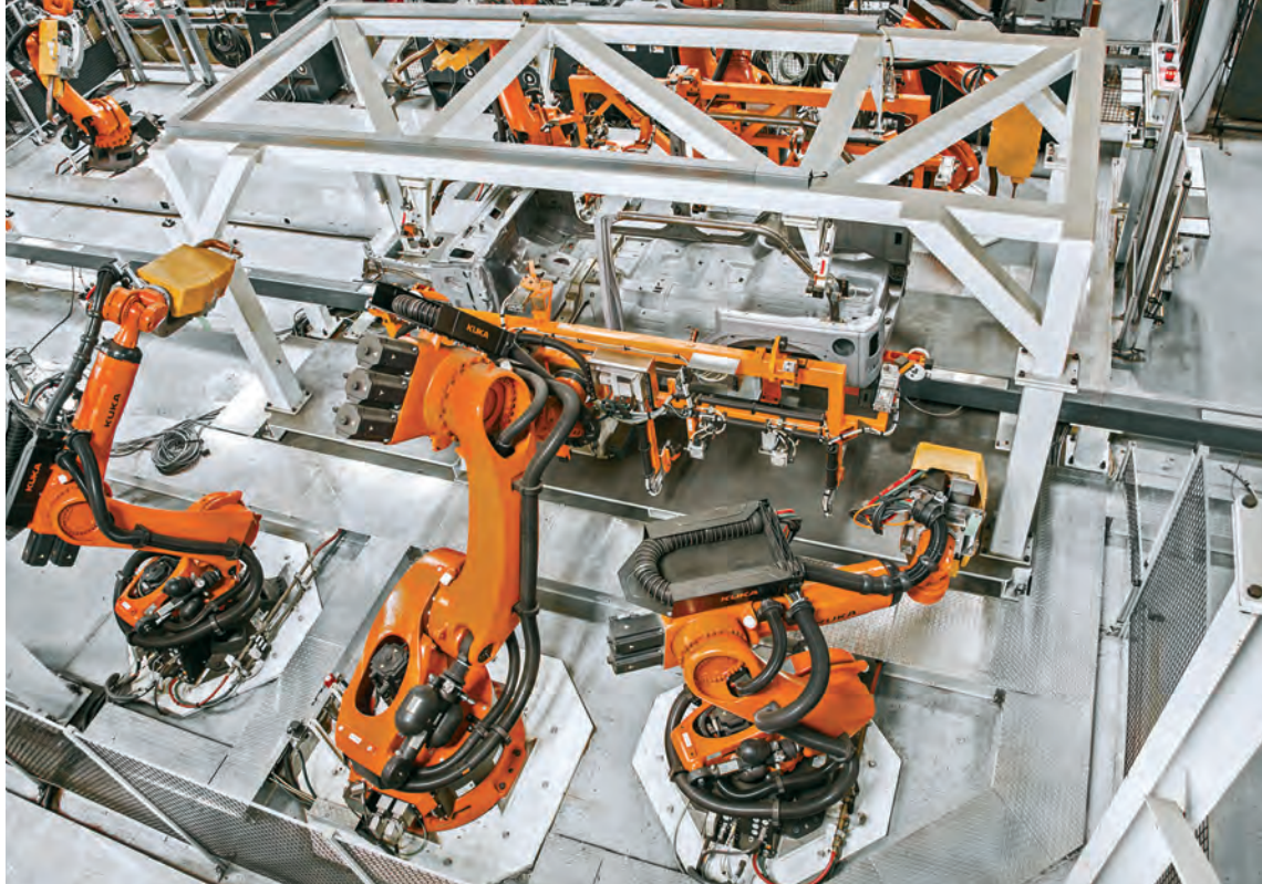
KS Pulse moves vehicle body sections through robotic work cells.
