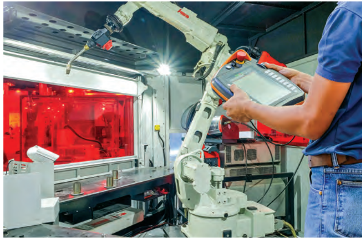
Operating a robotic welder.
