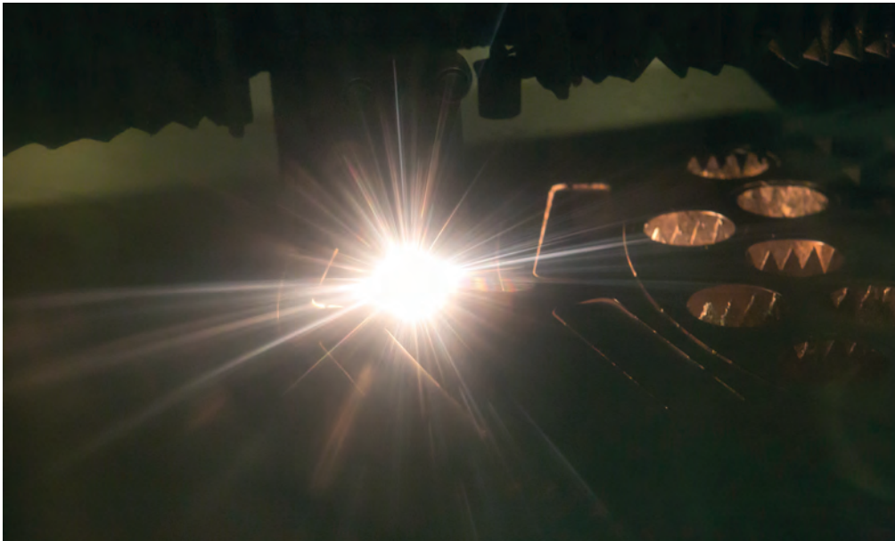
Cutting out the blades from sheets of high-quality steel.
