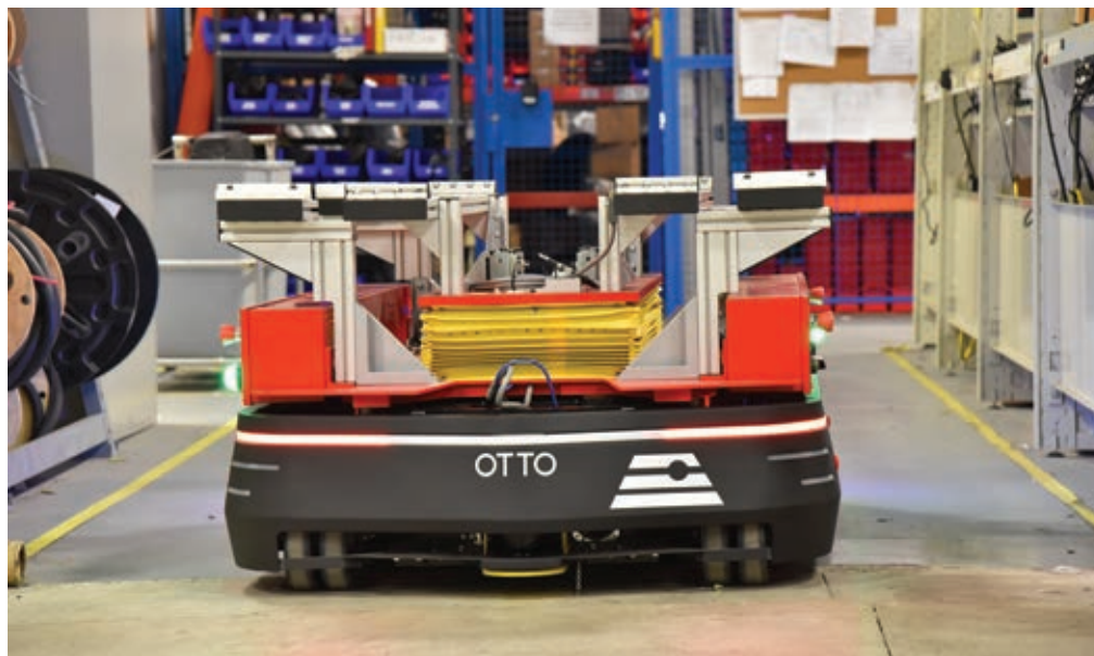
The OTTO 1500 self-driving vehicle performs tests with a lift and lower appliance.
