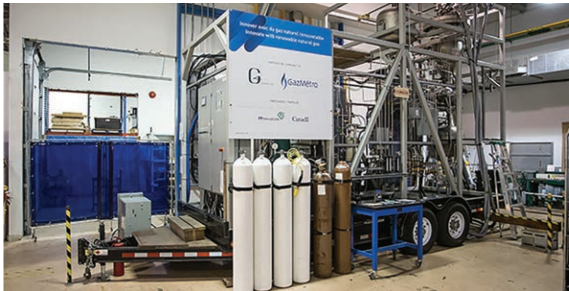
Gaz Metro's pilot project uses a thermochemical process to turn forest biomass into natural gas.
