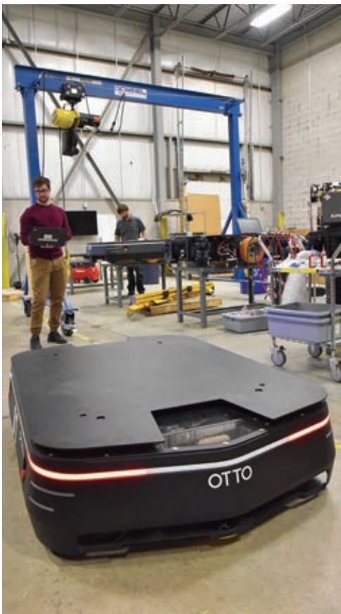
An OTTO Motors team member maps the facility using the vehicle's LIDAR sensors.
