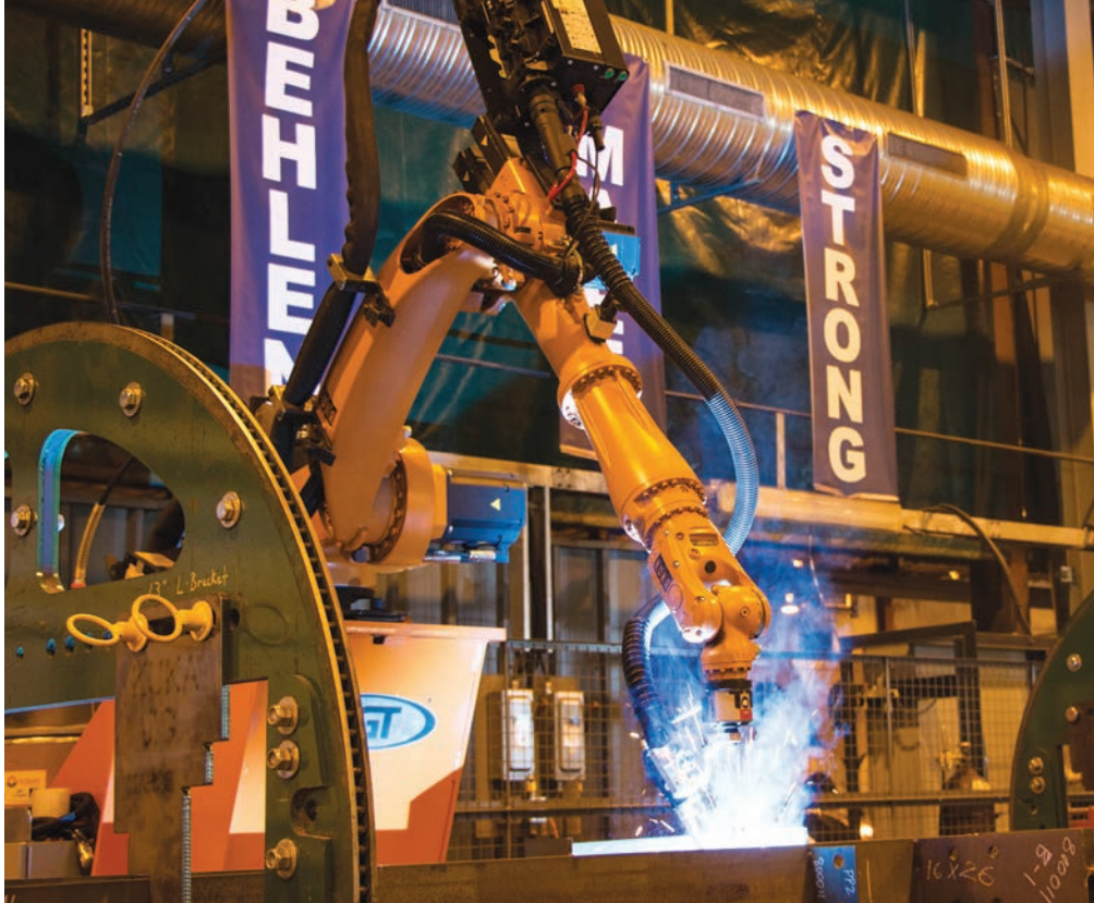
Behlen's robotic welder in action, improving quality and boosting capacity.
