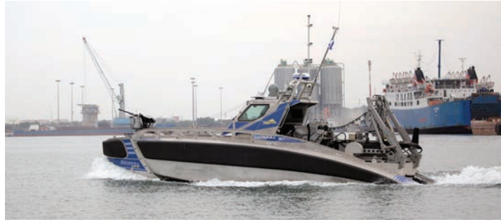
The Seagull USV from Elbit Systems can be fitted with Kraken's KATFISH sonar payload for remotely operated mine countermeasures and underwater intelligence.
