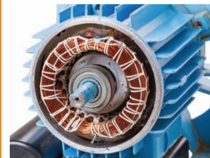
Low-temperature stripping spares the stator core.
