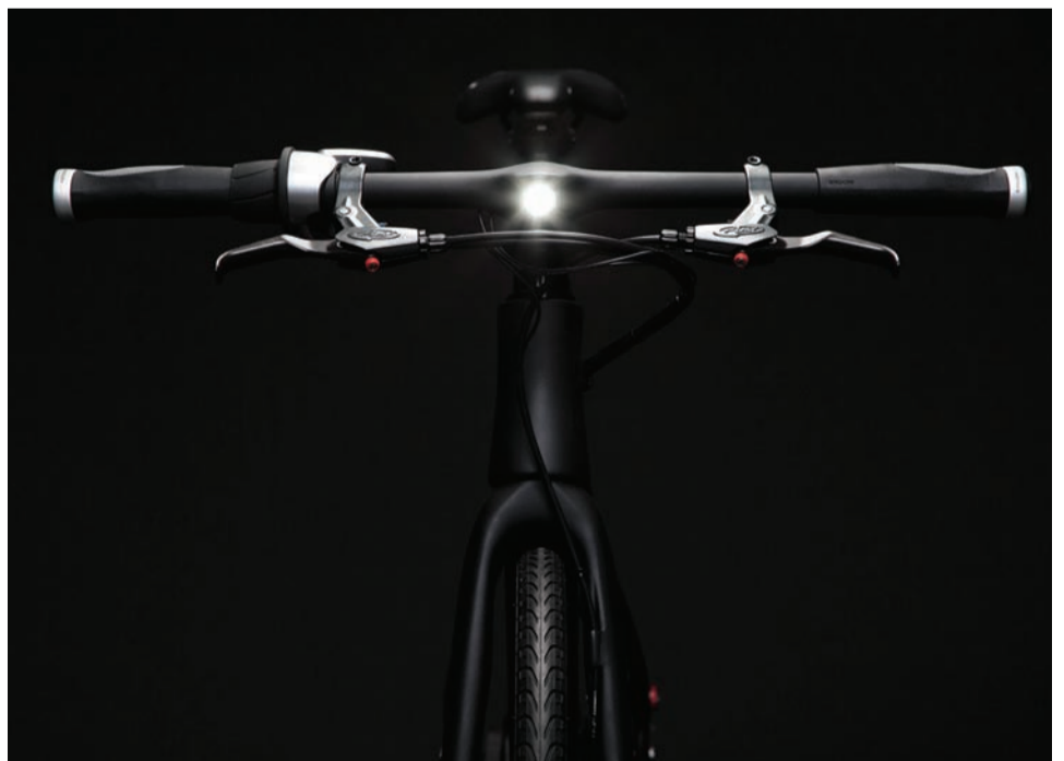
LED lights in the handlebars provide riders with hands-free, turn-by-turn GPS navigation.
