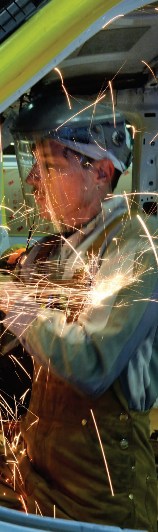
An INKAS employee grinds a vehicle's frame as part of the company's proprietary armouring process. PHOTOS: STEPHEN UHRANEY
