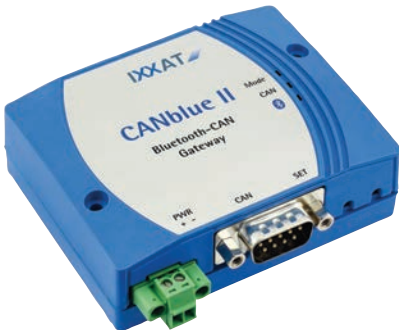
Connects CAN segments via Bluetooth.
