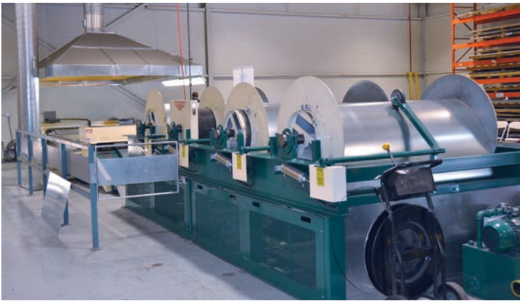
The new plasma feeder coil line replaces equipment that used standard-sized sheet metals, reducing the amount of wasted material.
