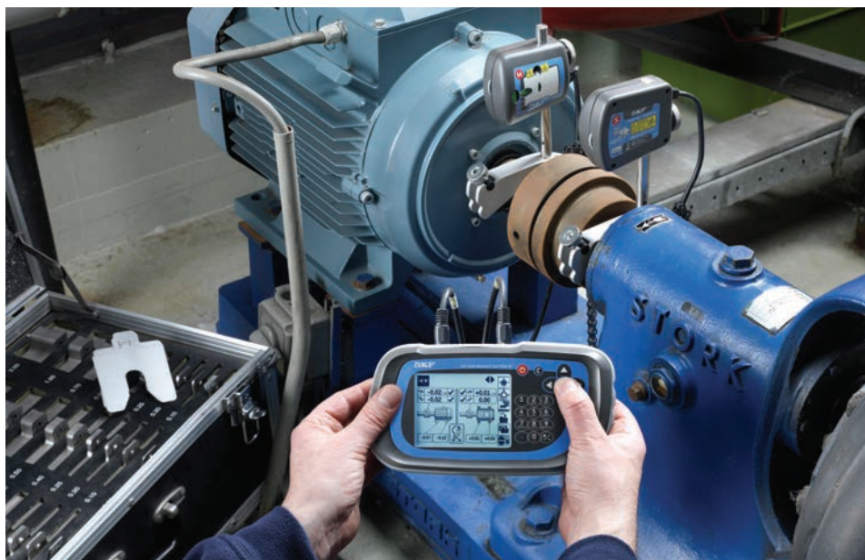
Shaft alignment systems with laser sighting reduce energy use.
