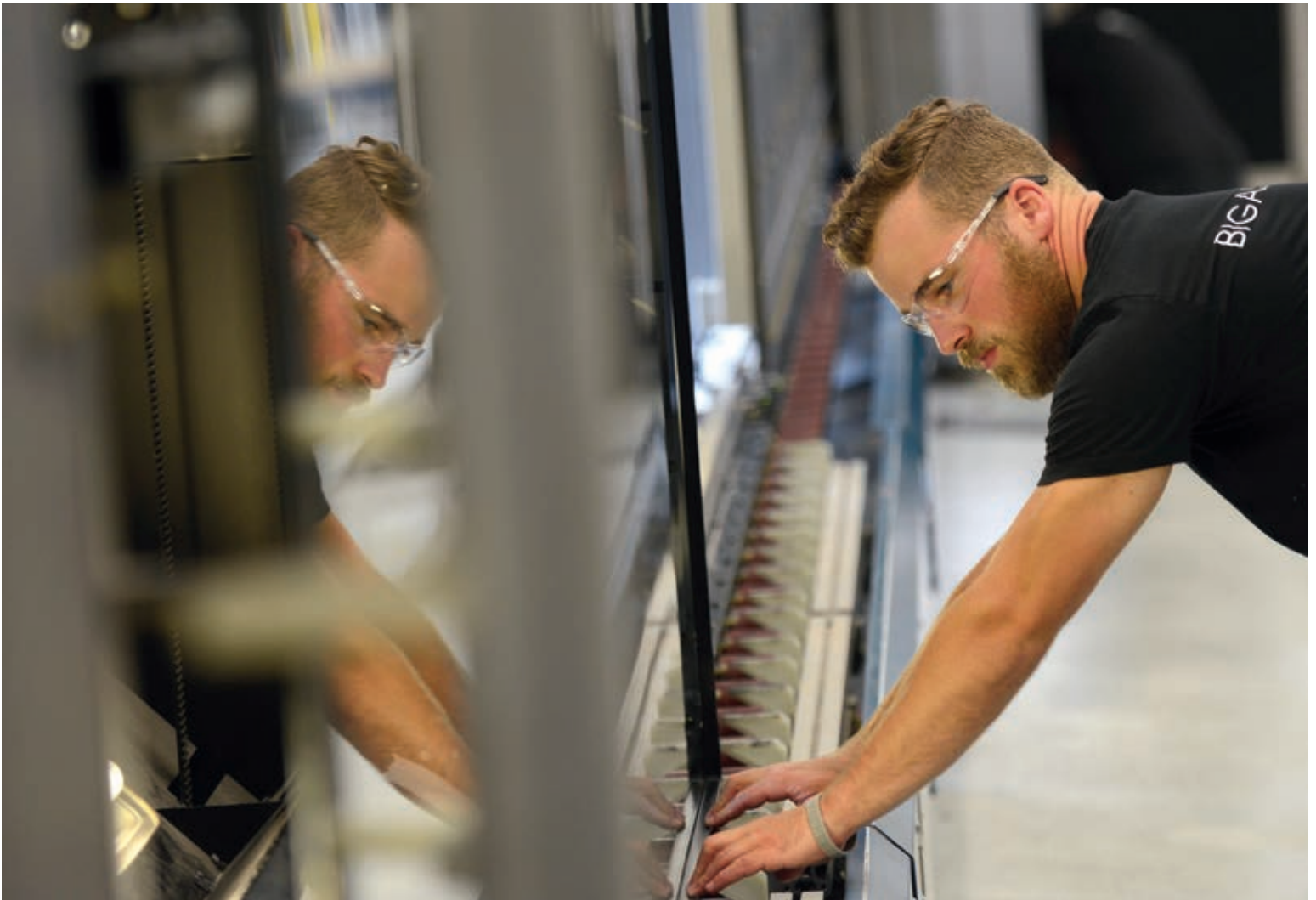
Cody Calahan sets stainless steel spacers on an insulated glass unit.
