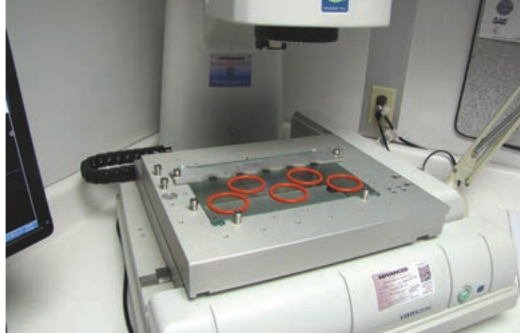
Newer digital devices take hundreds of measurements along the ID of the O-Ring for best accuracy.
